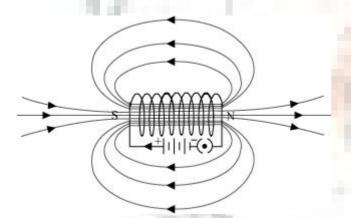
In the above figure, when the north pole of a bar magnet is brought near the end connected to the negative terminal of the battery, the solenoid repels the bar magnet. Since like poles repel each other, the end connected to the negative terminal of the battery behaves as the north pole of the solenoid and the other end behaves as a south pole. Hence, one end of the solenoid behaves as a north pole and the other end behaves as a south pole.
