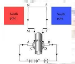
When a current is allowed to flow through the coil MNST by closing the switch, the coil starts rotating anti-clockwise. This happens because a downward force acts on length MN and at the same time, an upward force acts on length ST. As a result, the coil rotates anti-clockwise.
